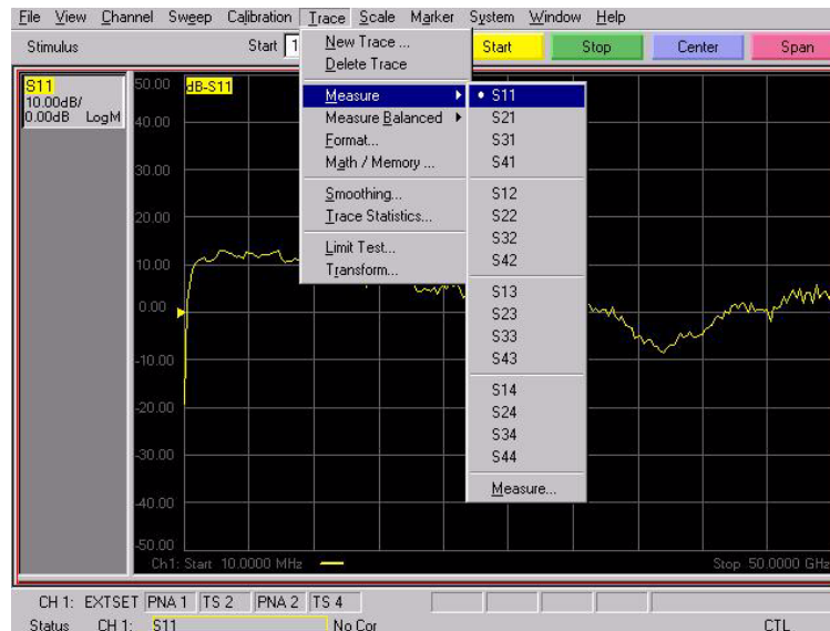
Figure 11 Checking for 4-Port Capability
